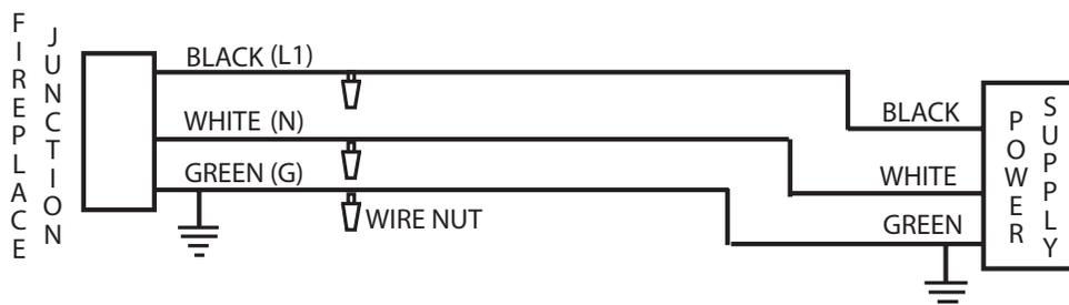
**NOTE:** To aid with moving the appliance, leave enough wire so that the log set can be removed from the enclosure without disconnecting the power supply. If servicing, shut off power supply.
