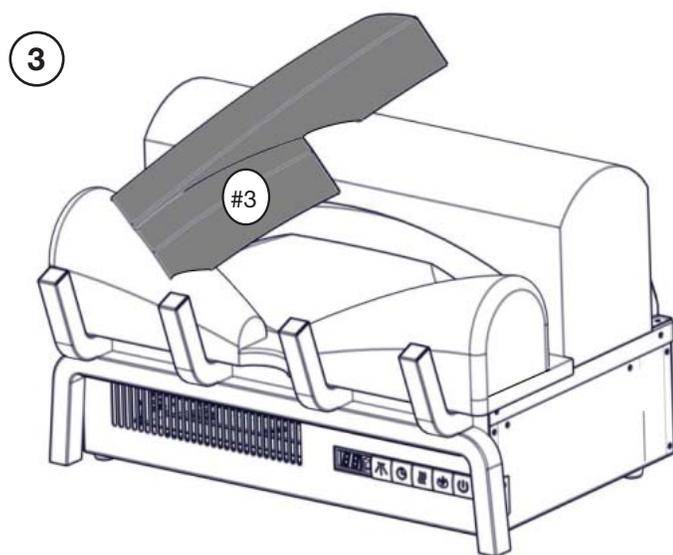
Place the log (#3) into the groove. Ensure the log is secure, as shown.
